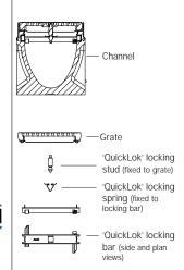
ACO 'QuickLok' is a patented boltless locking system, grates are removed and replaced with the minimum time and effort for ease of maintenance. The unique design provides a positive 'snap down' fit into the locking bar. A stud is fixed to the grate which 'locks' into the spring clip in the locking bar.
